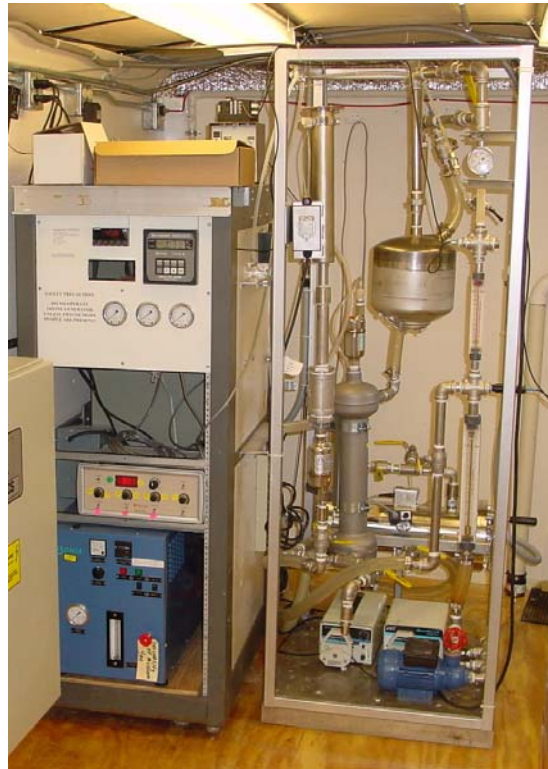
Figure II-12. Ozone/peroxide advanced oxidation process.
