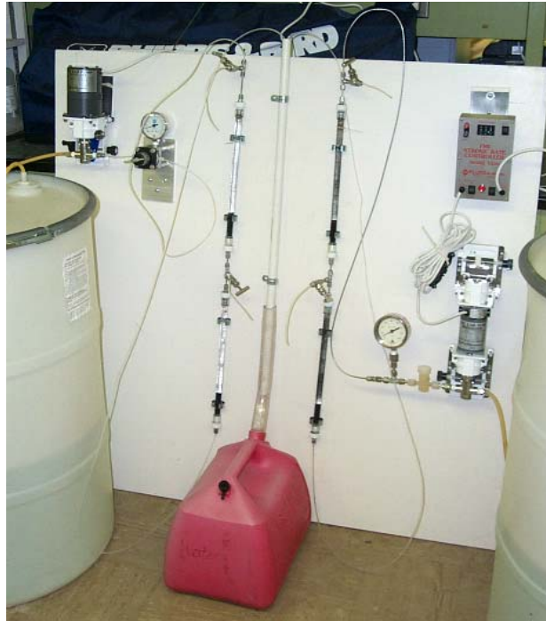
Figure II-7. Two RSSCT systems set up with two columns each in series.
