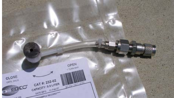
Fig 3: Connect transfer piece to tedlar bag.
