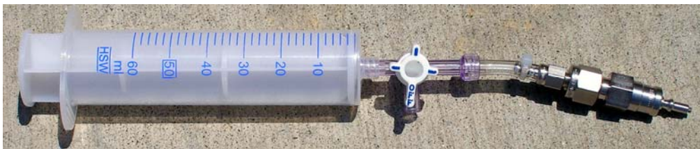
Fig 5: Flushing transfer piece
