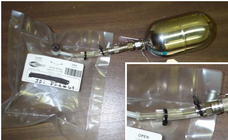
Fig 4: Connect summa to the tedlar with the transfer piece.
