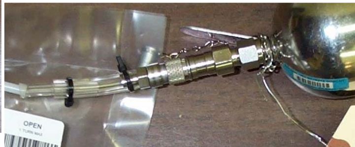
Fig 4: Connect summa to the tedlar with the transfer piece.
