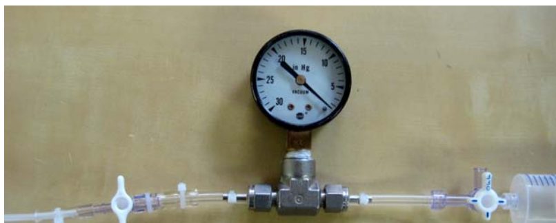
Fig 1: Attach syringe & vacuum gauge to soil gas probe tubing using 2-way & 3-way valves. Be sure to zip tie the connections.
