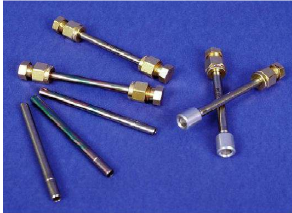
Adsorbent inside tube open on one end
